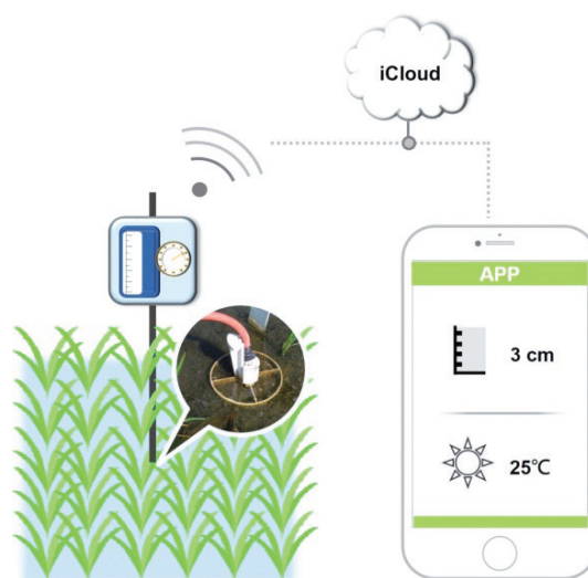
Fig. 2. Intelligent agriculture: received information of environmental factors by intelligent sensor in the field with internet.
